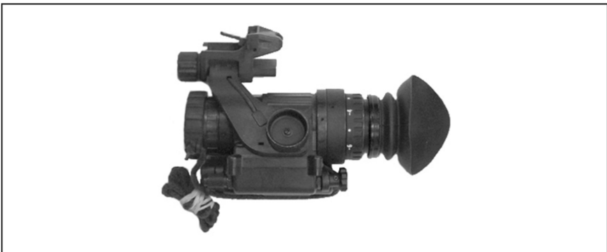
Figure 2-25. AN/PVS-14 Mounted With Helmet Clip
